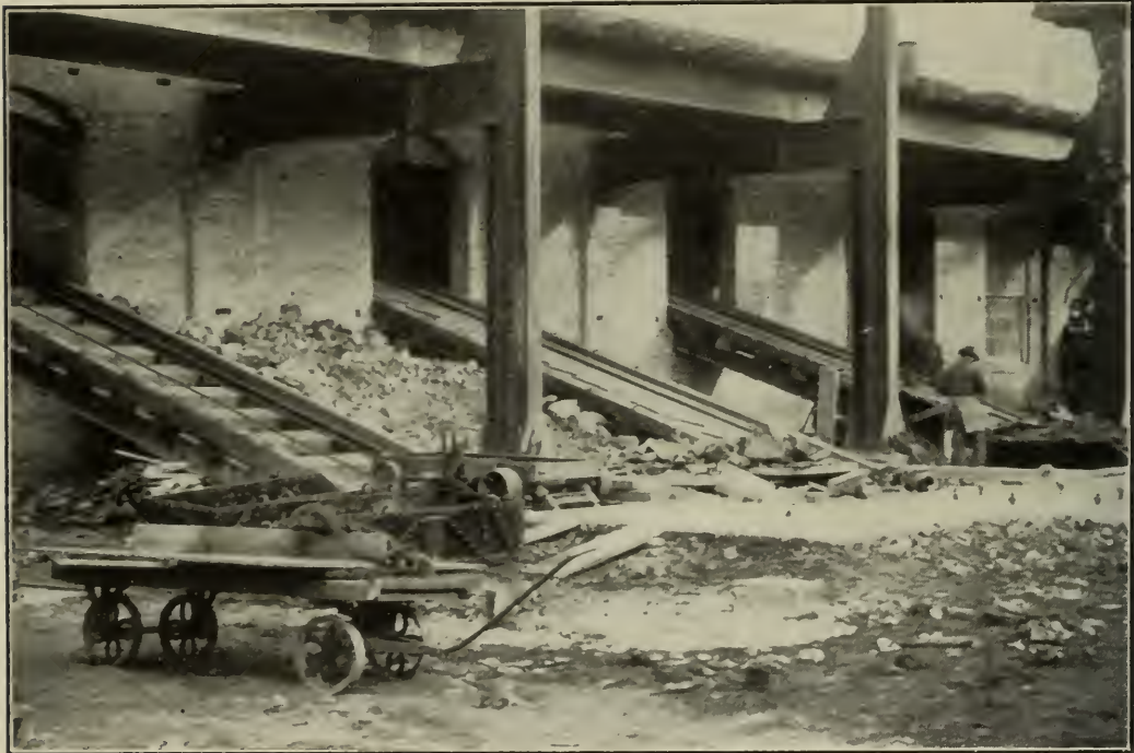
LOWER END OF SKIP INCLINE FOR CUPOLA-CHARGING APPARATUS, WEST ALLIS FOUNDRY OF ALLIS-CHALMERS COMPANY.
